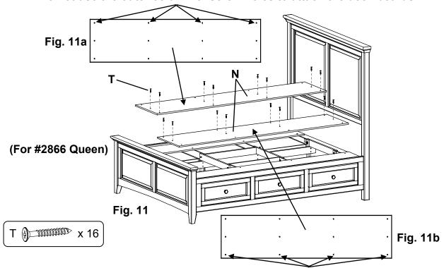
Do not use the outer column of screw holes to attach the deck boards
