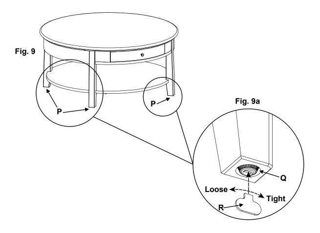
10. Place the table at its final destination. Use the Leveler Adjustment Key (R), found in the Zip bag taped to the Owner's Manual and Safety Guide to rotate the Slotted Levelers (Q) on the bottoms of the legs until the table is level. See Figures 9 and 9a.
