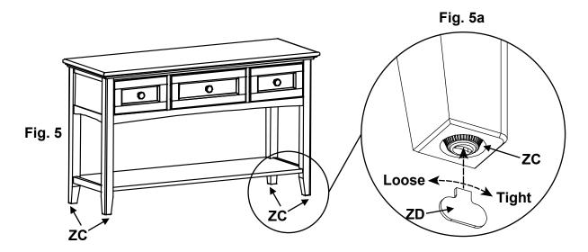
6. Place the table at its final destination. Use the Leveler Adjustment Key (ZD), found in the Zip bag taped to the Owner's Manual and Safety Guide to rotate the Slotted Levelers (ZC) on the bottoms of the legs until the table is level. See Figures 5 and 5a.
