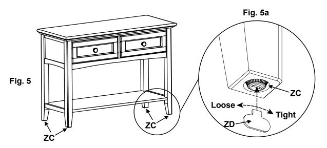
6. Place the table at its final destination. Use the Leveler Adjustment Key (ZD), found in the Zip bag taped to the Owner's Manual and Safety Guide to rotate the Slotted Levelers (ZC) on the bottoms of the legs until the table is level. See Figures 5 and 5a.
