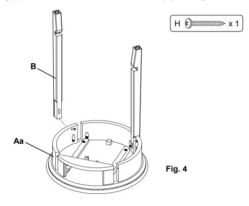
5. Place a third Leg (B) in a corner of the Top Assembly (Aa) and using the pocket hole as a guide, secure the Leg (B) with one #8 x 1-1/4" Pan Head Screw (H). See Figure 5.
