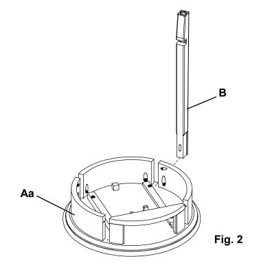
3. Using the pocket hole as a guide, secure the Leg (B) to the Top Assembly (Aa) with one #8 x 1-1/4" Pan Head Screw (H). See Figures 3 and 3a.
