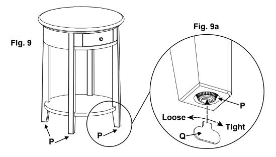
10. Place the table at its final destination. Use the Leveler Adjustment Key (Q), found in the Zip bag taped to the Owner's Manual and Safety Guide to rotate the Slotted Levelers (P) on the bottoms of the legs until the desk is level. See Figures 9 and 9a.
