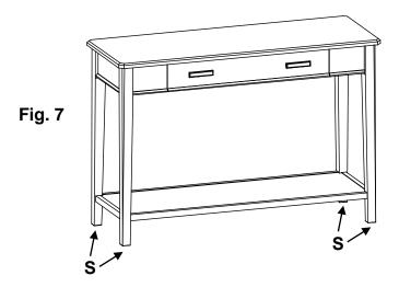
8. Place the table at its final destination. To level the table, rotate the Adjustable Glides (S) found on the bottoms of the legs. See Figure 7.
