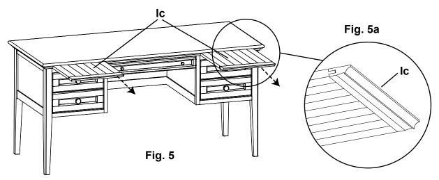
6. The center drawer can be used as a keyboard tray or utility drawer. To use it as a keyboard tray, open the drawer and pull down on the front. This unlocks the roller catches. To lock it back into place, push up on the drawer front.
