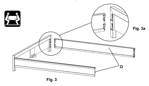
4. Align the Brackets on both sides and slide the Side Rail/Footboard assembly down on to the Headboard (A). See Figure 4.
