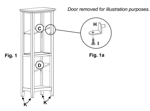
2. Place the tower at its final destination. Rotate the Adjustable Glides (K) found at the corners of the unit until the unit is level. See Figure 1.
