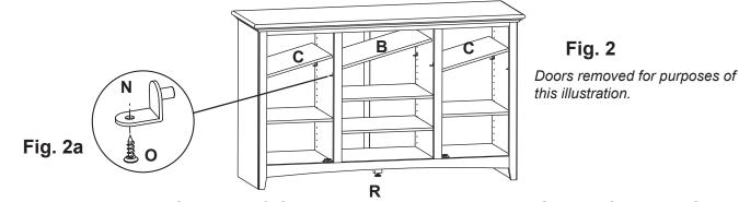
To move the Adjustable Shelves (B & C), remove the #6 x 1/2" Undercut Screws (O) and the Shelves (B & C). Reposition the Shelf Brackets (N) to the desired positions, replace the shelf and insert the screws. See Figures 2 and 2a.
