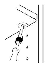
Position the screwdriver at a 25° angle.
