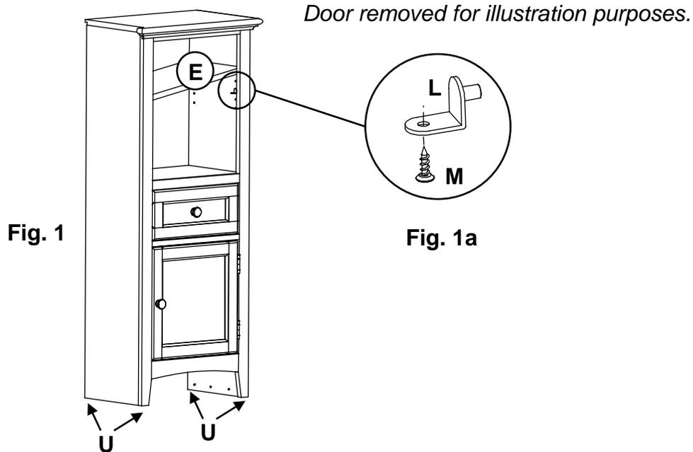
2. Move the piers to your desired location. To level the piers, rotate the Adjustable Glides (U) found on the bottoms of the legs. See Figure 1.
